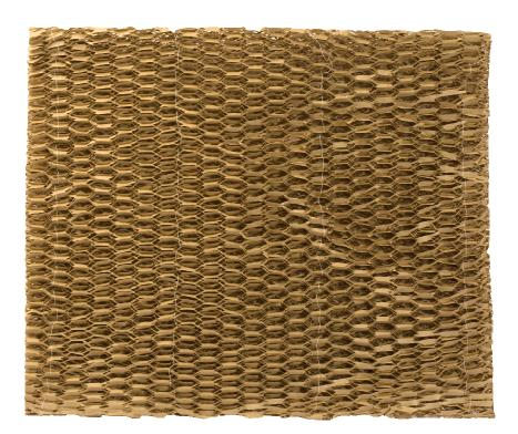
Cross section: Larger opening in the front; progressively smaller diamonds in the back of the filter
