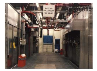
VOLVO AERO in Trollhättan, A-workshop, (pictures above). Flaw detection of aeroplane engine parts in an automatic installation. The goods are loaded in baskets transported through the installation by a "Power and free" conveyor. Step interval can be chosen between 15, 30 or 60 minutes. The following stations are included: - Loading.
