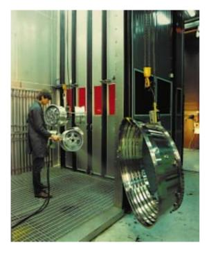
VOLVO AERO in Trollhättan, A-workshop. Penetrant flaw detection of aeroplane parts in a manually operated installation. This is a solution for less numbers of larger components. All the steps here are performed manually and everything apart from the final inspection takes place in one room. Ventilation is horisontical and the booth is a cascade curtain.
